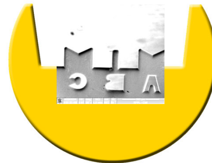
TEM sample "grid", diameter 3mm
